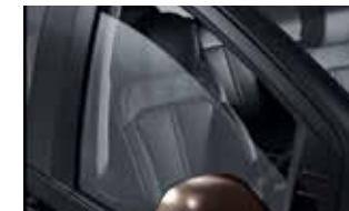
1st-row Double-laminated Soundproof Glass
